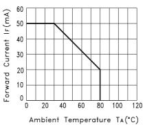
Fig.3 Forward Current Derating Curve
