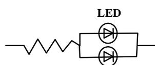
(B) The brightness of each LED might appear different due to the differences in the I-V characteristics of those LEDs.
