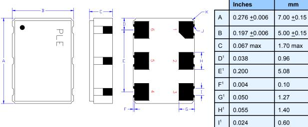
Contacts: Gold 11.8 µinches 0.3 µm minimum over Nickel 50 to 350 µinches 1.27 to 8.89 µm
