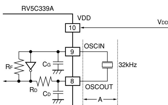
Typical externally-equipped element
