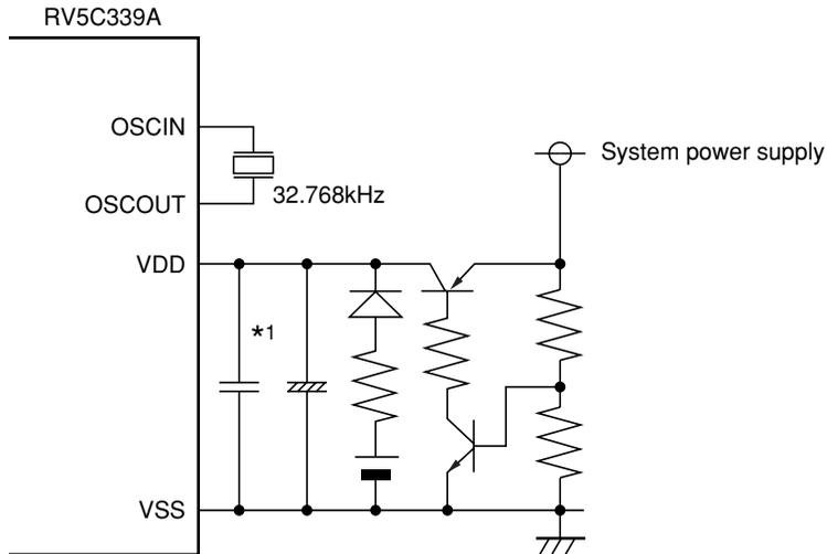
\*1) Install bypass capacitors for high-frequency and low-frequency applications in parallel in close vicinity to the RV5C339A.
