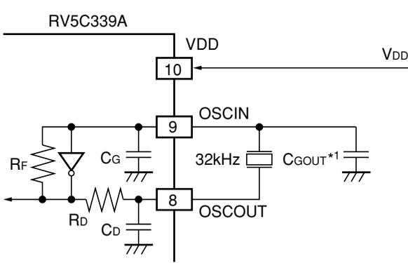
\*1) The CGOUT should have a capacitance ranging from 0 to 15pF.
