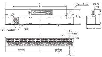
Note: There is only one DIN Track lock located in the center of the terminal block for a 20-pole Unit.
