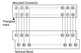
Note: For all models, the odd-numbered pins on the Connector correspond to row A on the terminal block and the even-numbered pins on the Connector correspond to row B on the terminal block.
