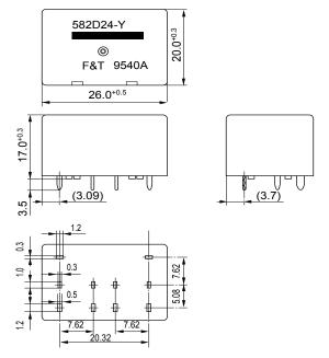
PC board mounting hole layout (BOTTOM VIEW)
