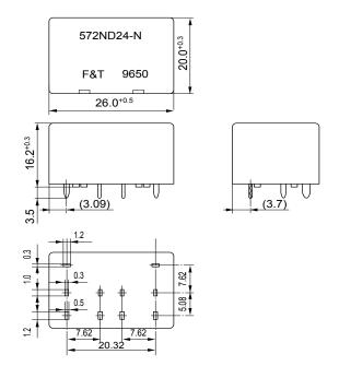
PC board mounting hole layout (BOTTOM VIEW)
