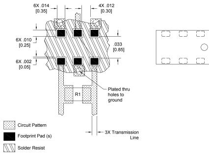
Dimensions are in Inches [Millimeters] Mounting Footprint
