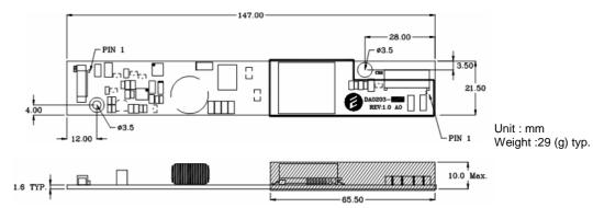
Note: Please use plastic screw in case of a non-insulating mounting base!
