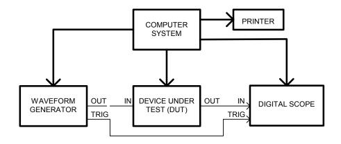
Figure 2: Test Setup
