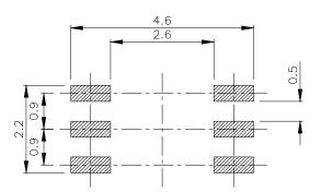
**Notes:** 1.All dimensions are in millimeters. 2.Tolerances unspecified are  $\pm 0.1$ mm.
