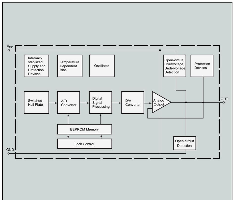
Fig. 2: Block diagram of the HAL 880
