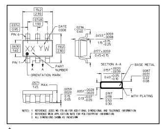
T Reference Application Note M538 for lead-free solder reflow recommendations. Meets JEDEC moisture sensitivity level 1 requirements.
