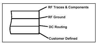
PCB dielectric between RF traces and RF ground layers should be chosen to reduce RF discontinuities between 50  $\Omega$  lines and package pins. M/A-COM recommends an FR-4 dielectric thickness of 0.008" (0.2 mm) yielding a 50  $\Omega$  line width of 0.015" (0.38 mm). The recommended metallization thickness is 1 oz. Copper.
