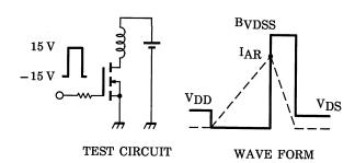
$$\begin{aligned} R_G &= 25 \ \Omega \\ V_{DD} &= 90 \ V, \ L = 12.2 \ mH \end{aligned} \qquad E_{AS} = \frac{1}{2} \cdot L \cdot I^2 \cdot \left( \frac{B_{VDSS}}{B_{VDSS} - V_{DD}} \right)$$
