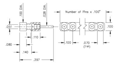
Description: Interconnect Header .100 Grid; Surface Mount Pin Header Horizontal Mount Single Row Surface Mount Plating Code: 10 Shell Plating: 10 μ" Gold over 100 μ" Nickel
