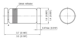
★ The gap between plug and glass can be either on cathode or anode side
