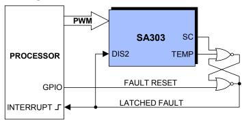
the device temperature falls below approximately 95°C. The TEMP pin hysteresis is wide to reduce the likelihood of thermal oscillations which can greatly reduce the life of the device.
