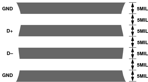
Figure 34. Typical Arrangement of Signal Tracks
