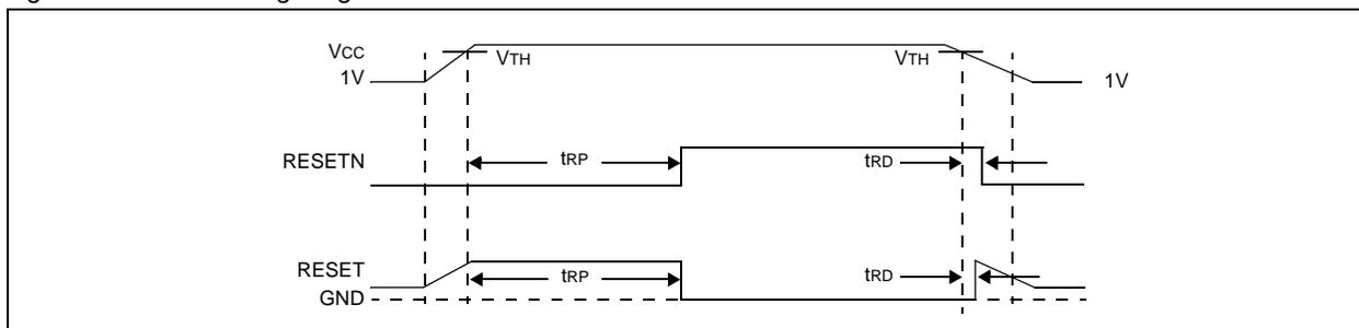
Figure 11. Functional Diagram of RESETIN Supervisory Application
