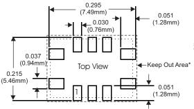
\* Do not route any traces in the keep out area. It is recommended the next layer under the keep out area is to be ground plane.
