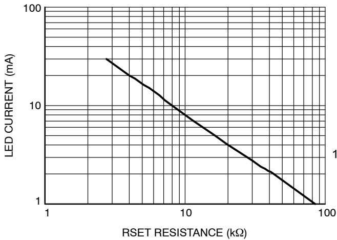
Figure 13. LED Current vs. RSET Resistance
