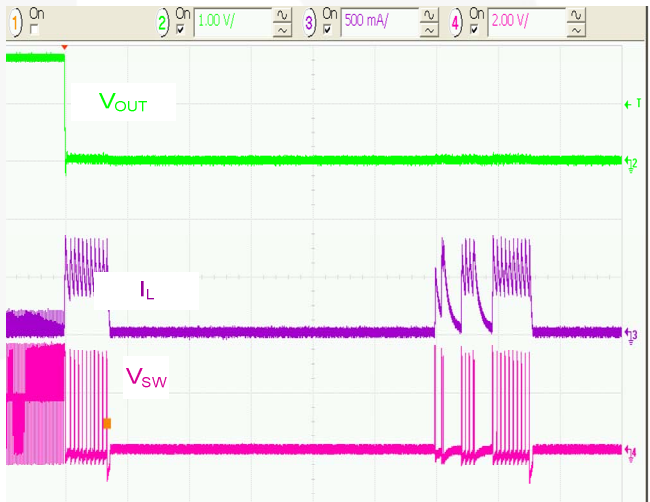
Figure 16. Metallic Short Applied at V OUT , 50 \mu s /div.
