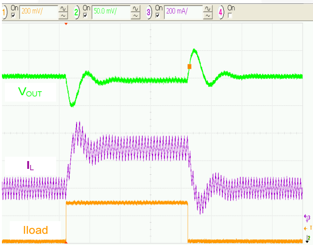
Figure 15. Load Transient 200 to 500mA, 3.6V IN , 5 \mu s /div.
