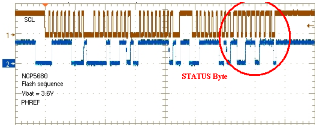
Figure 23. Basic I2C Read Sequence to Extract the STATUS Register
