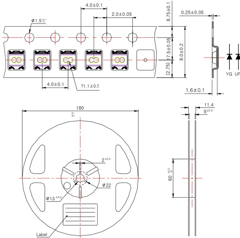
Tolerance: ±0.2, Unit: mm
