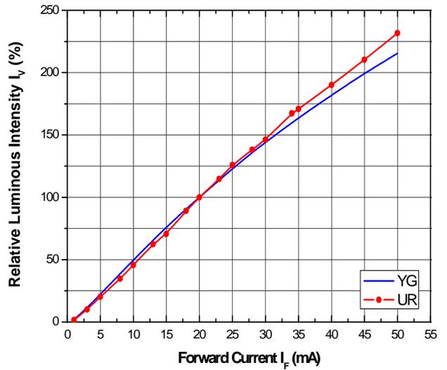
Forward Current vs Derating Curve
