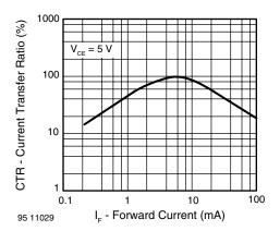
Fig. 11 - Current Transfer Ratio vs. Forward Current
