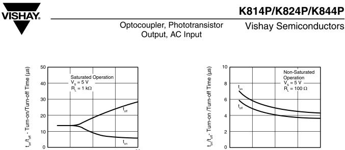
Fig. 12 - Turn-on/Turn-off Time vs. Forward Current
