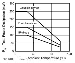
Fig. 4 - Total Power Dissipation vs. Ambient Temperature
