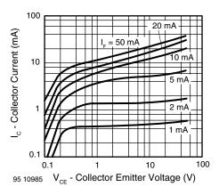
Fig. 9 - Collector Current vs. Collector Emitter Voltage
