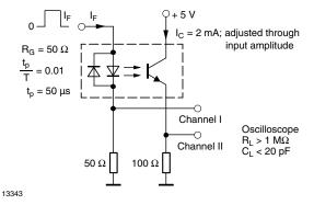
Fig. 1 - Test Circuit, Non-Saturated Operation
