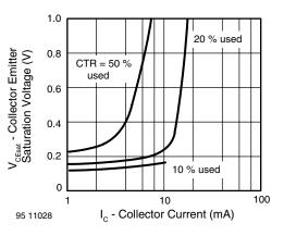
Fig. 10 - Collector Emitter Saturation Voltage vs. Collector Current
