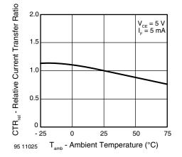
Fig. 6 - Relative Current Transfer Ratio vs. Ambient Temperature
