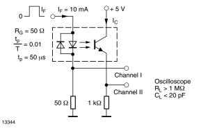
Fig. 2 - Test Circuit, Saturated Operation
