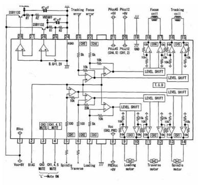
T.S.D : (Thermal shutdown) Resistance unit :  $[\Omega]$
