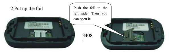
3 Insert SIM card into the holder, put down the foil right and fasten it.
