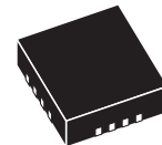
QFN16 (Q) 3 mm x 3 mm
