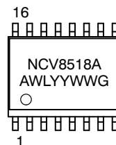
SOIC-16 LEAD WIDE BODY EXPOSED PAD CASE 751R
