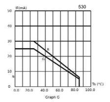
^ = Products must be derated according to the derating information. Each derating graph refers to specific LEDs.
