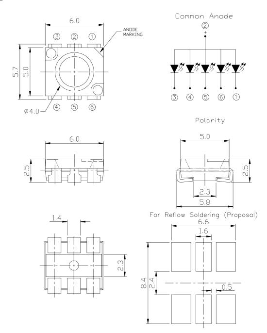
**Notes:** 1.All dimensions are in millimeters. 2.Tolerances unspecified are  $\pm 0.1$ mm.
