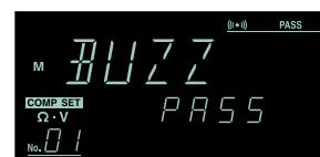
Buzzer mode setting
