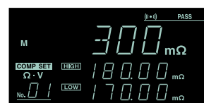
Resistance comparator value setting
