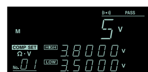
Voltage comparator value setting
