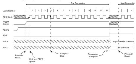
Figure 21-7. ADC Timing Diagram, Free Running Conversion
