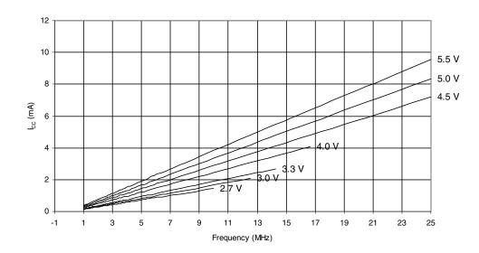
Figure 27-7. IIdle Supply Current vs. V<sub>CC</sub> (Internal RC Oscillator, 8 MHz)
