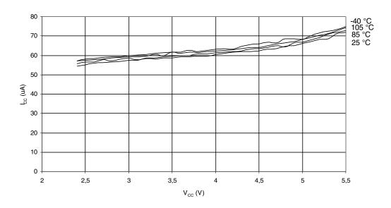
Figure 27-43. Programming Current vs.  $V_{\text{CC}}$
