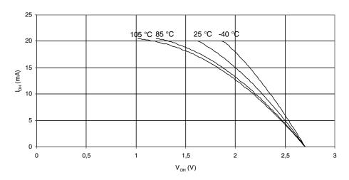
Figure 27-17. I/O Pin Sink Current vs. Output Voltage ( $V_{CC} = 5V$ )
