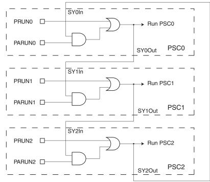
Figure 16-38. PSC Run Synchronization
