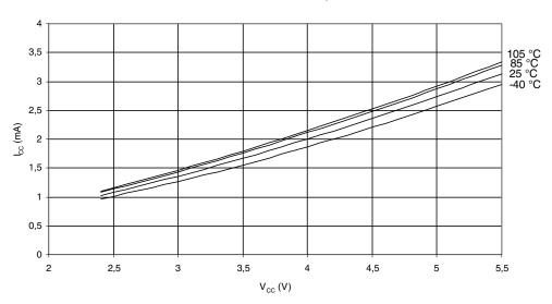
Figure 27-8. Idle Supply Current vs. V<sub>CC</sub> (Internal PLL Oscillator, 16 MHz)
