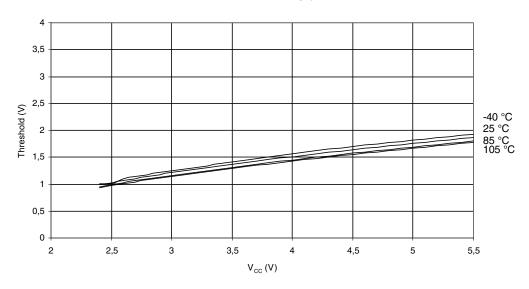
Figure 27-27. PE0 Input Threshold Voltage vs.  $V_{CC}$  (PE0 Pin Read As '1')
