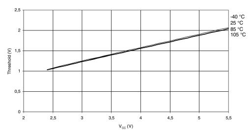
**Figure 27-20.** I/O Pin Input Threshold Voltage vs.  $V_{CC}$  (VIL, I/O Pin Read As '0') I/O PIN (including PE1 & PE2) INPUT THRESHOLD VOLTAGE vs.  $V_{CC}$  VIL, IO PIN READ AS '0'
