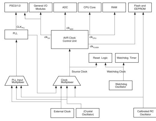
Figure 7-2. Clock Distribution AT90PWM2B/3B
