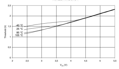
Figure 27-23. Reset Input Threshold Voltage vs.  $V_{CC}$  (VIL, Reset Pin Read As '0') RESET INPUT THRESHOLD VOLTAGE vs.  $V_{CC}$  VIL, RESET PIN READ AS '0'
