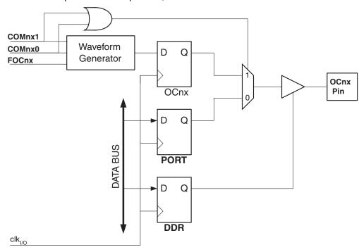
Figure 15-5. Compare Match Output Unit, Schematic
