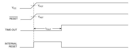
Figure 9-3. MCU Start-up, RESET Extended Externally
