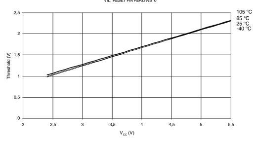
Figure 27-24. Reset Input Pin Hysteresis vs.  $V_{CC}$  RESET PIN INPUT HYSTERESIS vs.  $V_{CC}$
