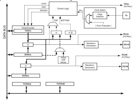
Figure 14-1. 8-bit Timer/Counter Block Diagram
