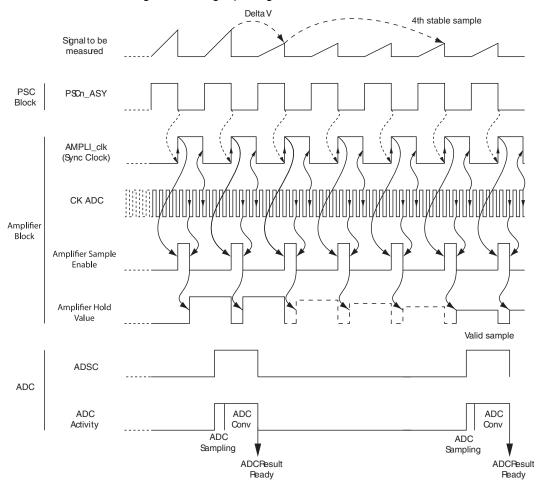
**Figure 21-16.** Amplifier synchronization timing diagram for AT90PWM2B/3B With change on analog input signal
