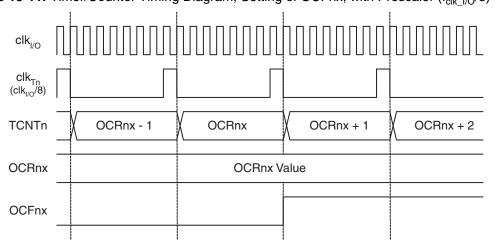
Figure 15-11. Timer/Counter Timing Diagram, Setting of OCFnx, with Prescaler (folk 1/0/8)
