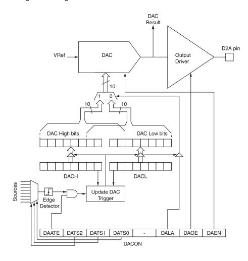
Figure 22-1. Digital to Analog Converter Block Schematic
