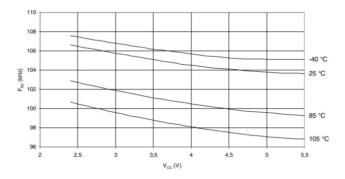
Figure 27-36. Calibrated 8 MHz RC Oscillator Frequency vs. Temperature
