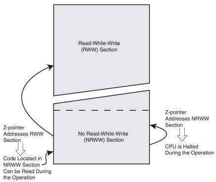
Figure 24-1. Read-While-Write vs. No Read-While-Write
