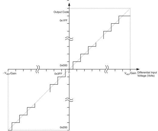
Figure 21-14. Differential Measurement Range
