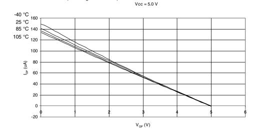
Figure 27-12. I/O Pin Pull-Up Resistor Current vs. Input Voltage ( $V_{CC} = 2.7V$ )
