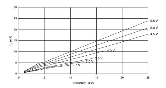
Figure 27-3. Active Supply Current vs. V<sub>CC</sub> (Internal RC Oscillator, 8 MHz)
