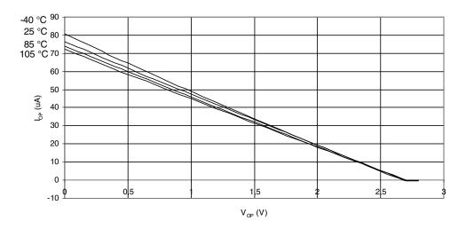
Figure 27-13. Reset Pull-Up Resistor Current vs. Reset Pin Voltage ( $V_{CC}$  = 5V) PE0 and RESET PULL-UP RESISTOR CURRENT vs. INPUT VOLTAGE  $V_{CC}$  = 5.0 V
