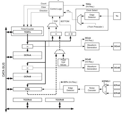
Figure 15-1. 16-bit Timer/Counter Block Diagram<sup>(1)</sup>
