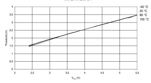
Figure 27-28. PE0 Input Threshold Voltage vs. V<sub>CC</sub> (PE0 Pin Read As '0')
