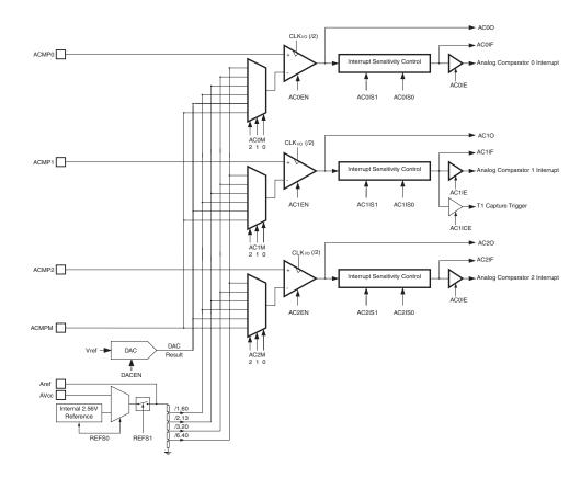
Figure 20-1. Analog Comparator Block Diagram<sup>(1)(2)</sup>
