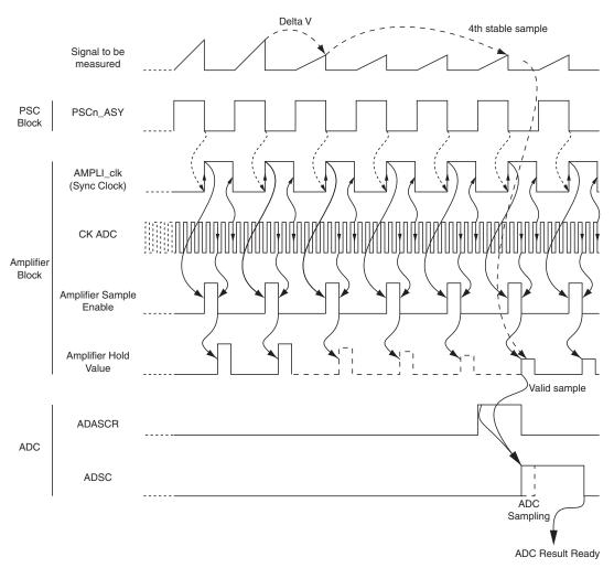
It is also possible to auto trigger conversion on the amplified channel. In this case, the conversion is started at the next amplifier clock event following the last auto trigger event selected thanks to the ADTS bits in the ADCSRB register. In auto trigger conversion, the free running mode is not possible unless the ADSC bit in ADCSRA is set by soft after each conversion.
