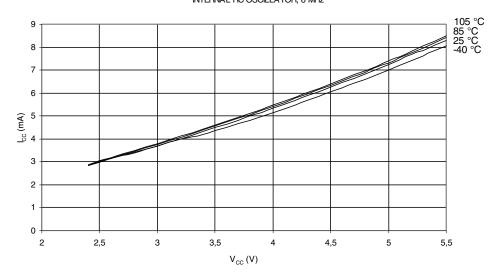
$\textbf{Figure 27-4.} \quad \text{Active Supply Current vs. V}_{\text{CC}} \text{ (Internal PLL Oscillator, 16 MHz)}$
