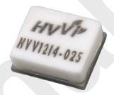
The device resides in a Surface Mount Transistor Package with a ceramic lid. The SM200 package style is qualified for gross leak test – MIL-STD-883, Method 1014.
