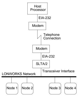
An adapter implemented with the LTS-10 module supports the LonTalk network management messages for controlling an attached modem. Any node can initiate an outgoing call to a remote host by sending network management dialing messages to the adapter. Network management messages can be used to define a dialing directory stored in the adapter, enabling application nodes to dial out to remote hosts without requiring host phone numbers to be maintained in every node.
