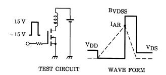
$$\begin{aligned} &RG=25~\Omega\\ &V_{DD}=90~V,~L=8.3~mH \end{aligned} \qquad EAS$$
