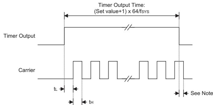
**Timer Output when Carrier Is an Output**
