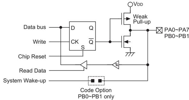
PA, PB0~PB1 Input/Output Lines
