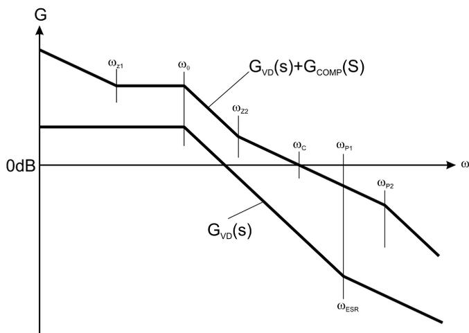
Fig2. Power stage and compensated loop gain.
