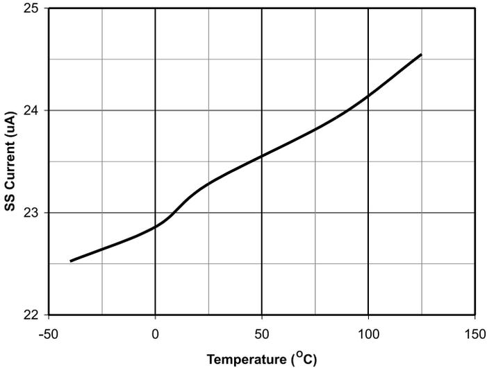
Typical Error Amp Output Current vs Temperature
