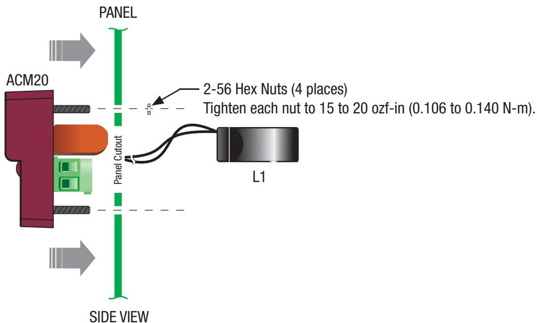
Figure 5. Panel Installation
