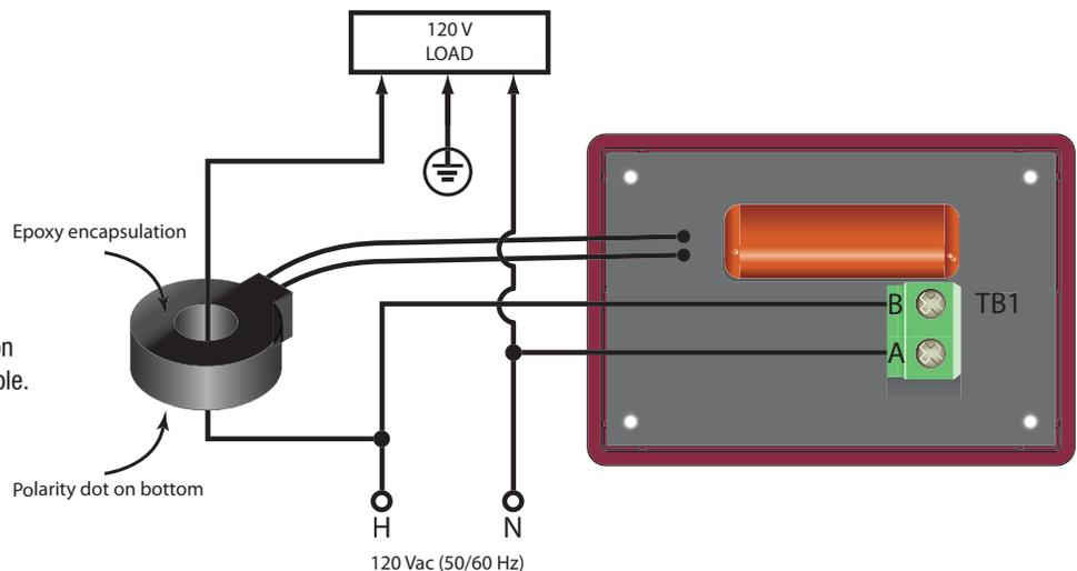
Figure 1. Wiring diagram for 110/120V single phase systems
