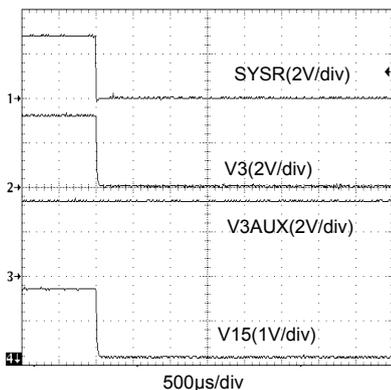
Fig.10 Power Down Wave Form (Active to Standby)
