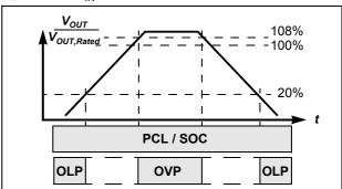
Figure 7 V<sub>OUT</sub> Related Protection Features
