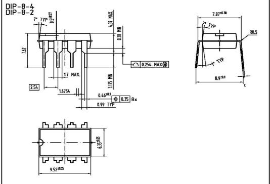
Figure 17 PG-DSO-8 and PG-DIP-8 Outline Dimension
