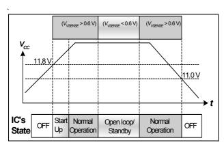
Figure 3 State of Operation respect to VCC
