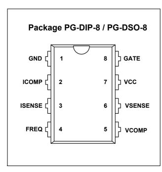
Figure 1 Pin Configuration (top view)
