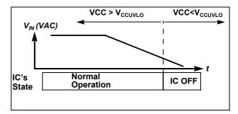
Figure 6 V<sub>IN</sub> Related Protection Features
