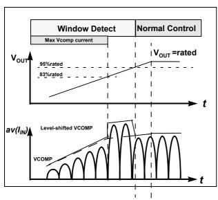
Figure 5 Startup with controlled maximum current
