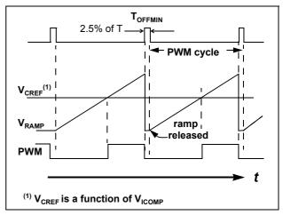
Figure 13 Ramp and PWM waveforms
