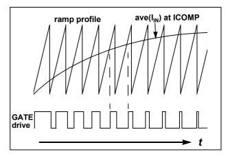
Figure 12 Average Current Control in CCM
