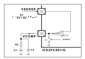
Figure 4 Startup Circuit
