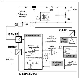
Figure 11 Complete System Current Loop
