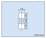
The recommended thickness of the screen mask for soldering is more than 150 $\mu m$ . The hole size of the screen mask should be same as the recommended land pattern or smaller.
