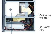
Shockproof disk drive housing for one 3.5" HDD and one slim-type optical drive
