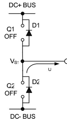
**Figure 13: D2 conducting**
