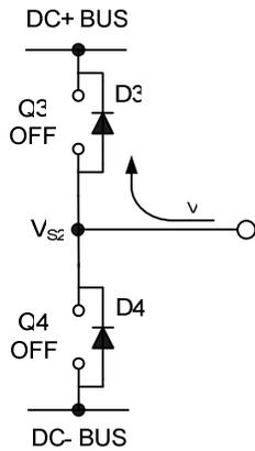
**Figure 14: D3 conducting**
