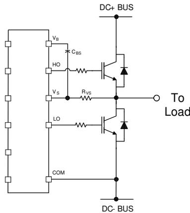
**Figure 22:  $V_S$  resistor**
