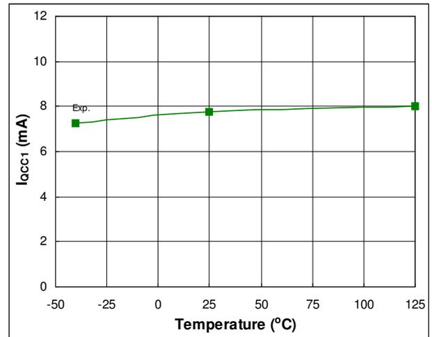
**Fig. 31. Quiescent VCC Supply Current vs. Temperature**
