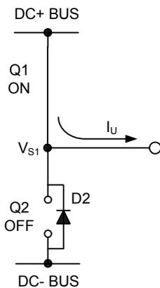
**Figure 12: Q1 conducting**
