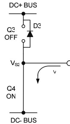
**Figure 15: Q4 conducting**
