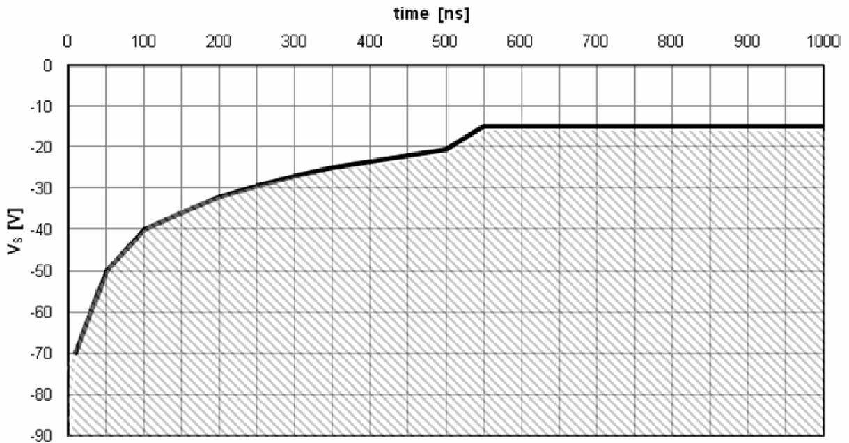
**Figure 19: Negative  $V_S$  transient SOA @  $V_{BS}=15V$**
