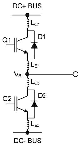
**Figure 16: Parasitic Elements**
