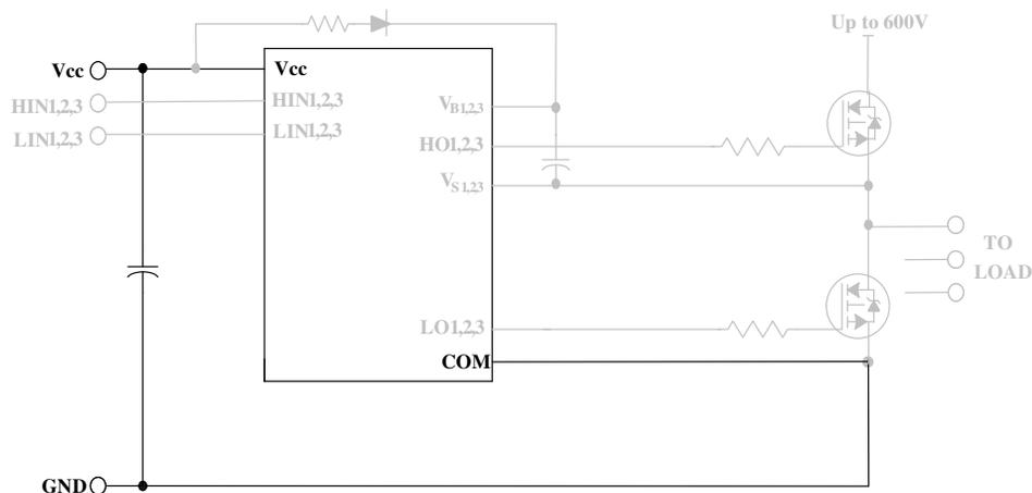
**Figure 21: Supply capacitor**
