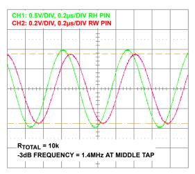
FIGURE 23. 10k -3dB CUT OFF FREQUENCY
