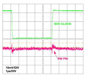
FIGURE 19. WIPER DIGITAL FEEDTHROUGH
