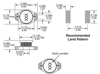
Part marking since Feb. 2005. Parts manufactured prior to that date may have color dots. Visit www.coilcraft.com/colrpowr.cfm for details.
