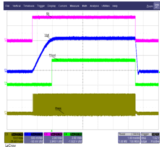
Ch1-Phase Voltage (10V/Div) Ch2-Vout(500mV/Div) Ch3-EN(2V/Div) Ch4-PGood(2V/Div)
