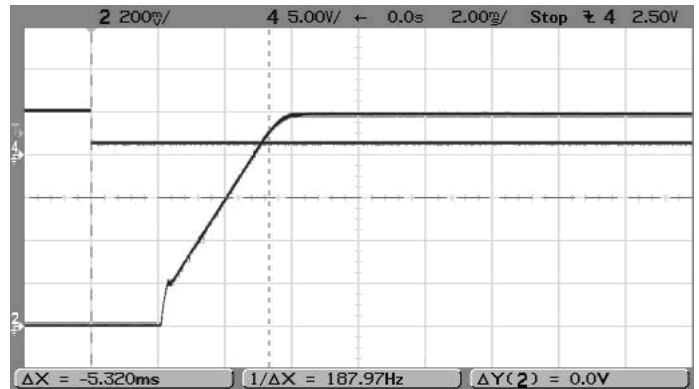
Step Load Transient Response (Vin=5V, Vout=1.0V, Clod=0, Iout=3A to 1.5A) Trace 2=Vout, 100 mV/div. Trace 4=Iout, 1A/div.
