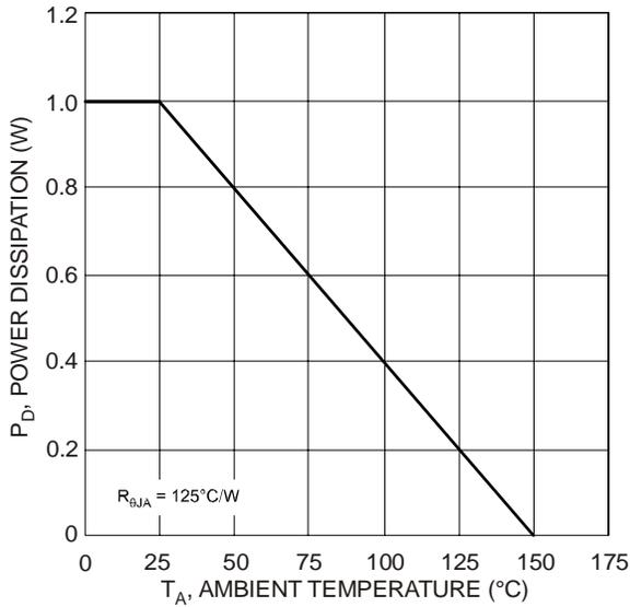
Fig. 1 Power Dissipation vs. Ambient Temperature (Note 3)
