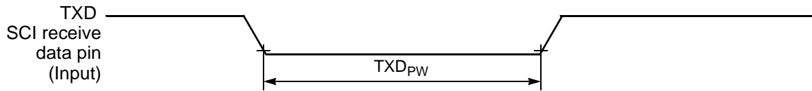
Figure 10-17 TXD Pulse Width
