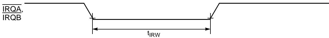
Figure 10-6 External Interrupt Timing (Negative Edge-Sensitive)
