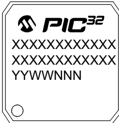
100-Lead TQFP (14x14x1 mm)
